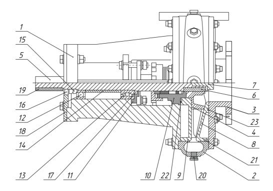
Centrifugal pump NC-350R1 (16"x14"x23"). Structure.
